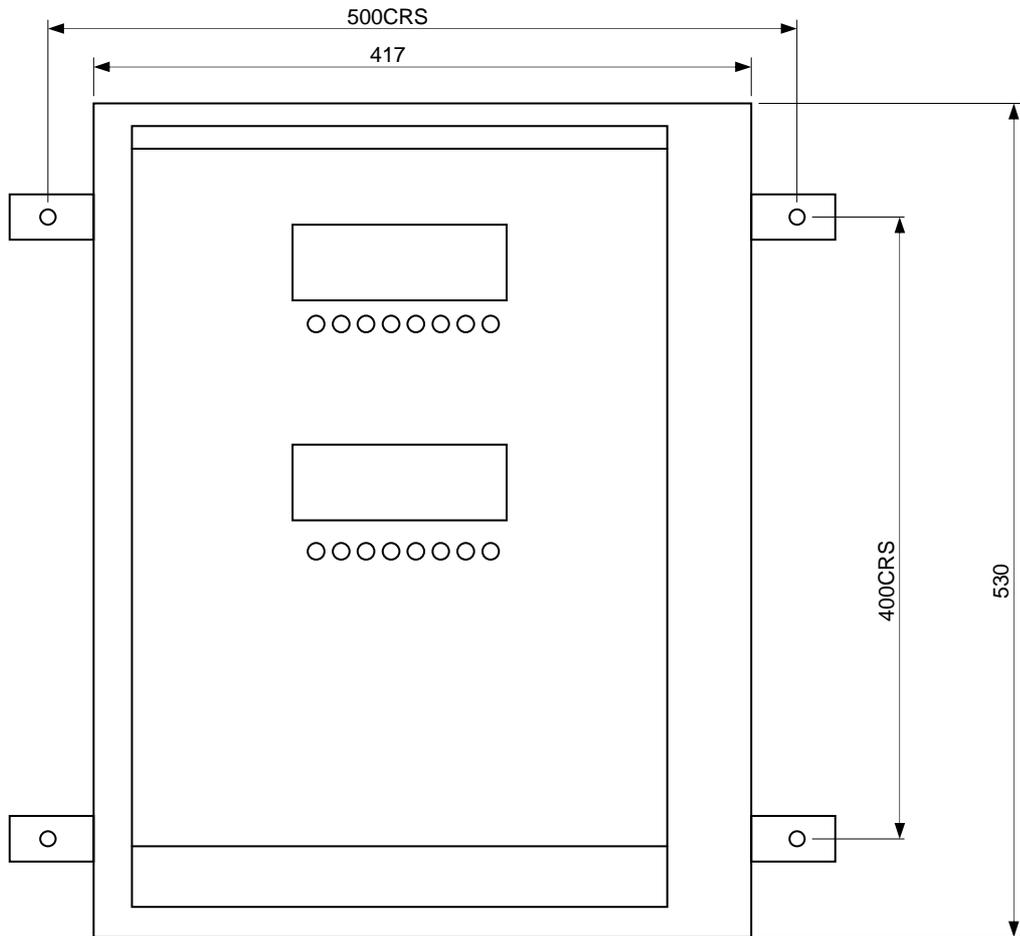
Four mounting holes are provided each having a diameter of 11mm.
