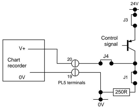
The SCM1 can provide a voltage output.
