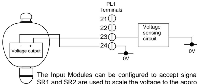
The Input Modules can be configured to accept signal levels in voltage form. SR1 and SR2 are used to scale the voltage to the appropriate level.
