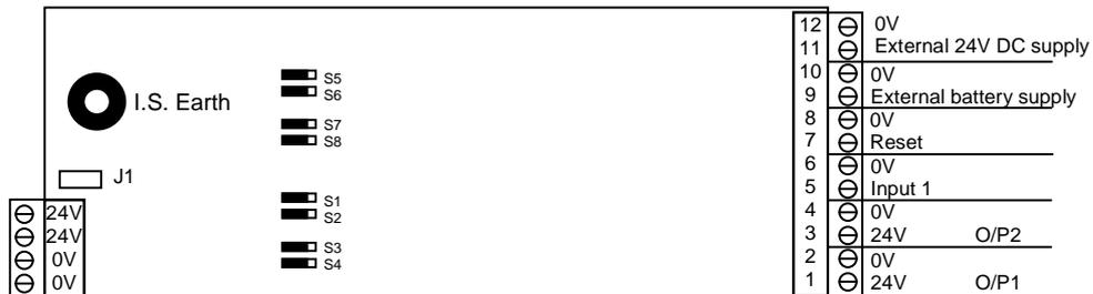
The lower 4-way connector provides two 24V screw terminals, and two 0V screw terminals. The voltages are always present at these terminals whilst FS3 is intact. This supply is taken from the 24V supply of the system and is used by Analox Ltd when powering external equipment. The amount of power available from this connector must be determined for each installation based upon the system configuration.
