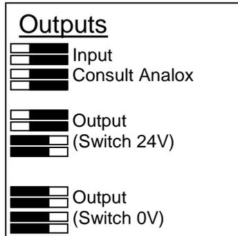
**Input** – Allows the outputs to be configured as inputs in some circumstances. Contact Analox Ltd for further details.
