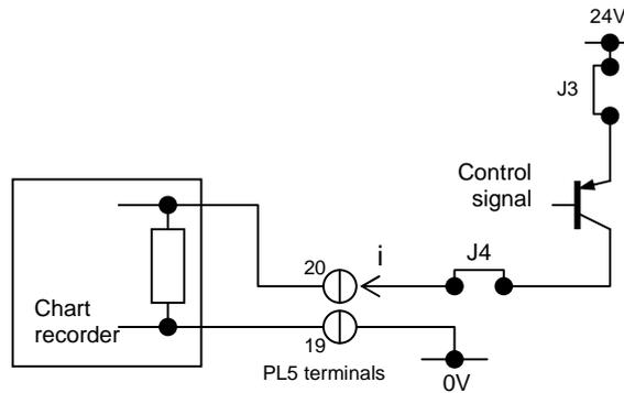
The input module sources current proportional to the detected gas level.
