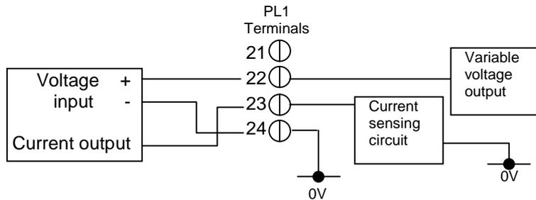
This configuration allows the connection of a detector head that provides a 4-20mA current output, and requires a separate power source, between 0 to 24V.
