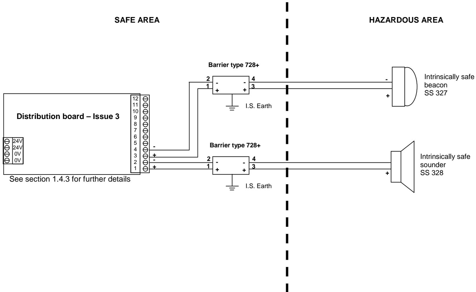
8.3 Example of connection to a Analox Ltd traffic light unit
