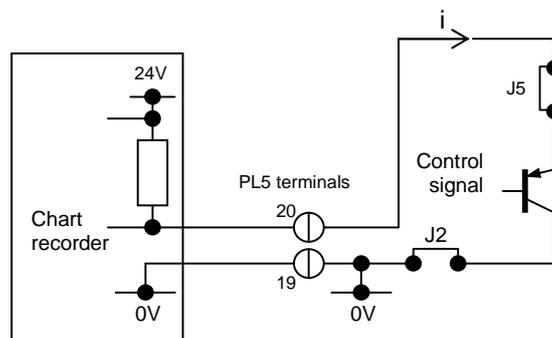
The input module can also sink current proportional to the detected gas level.
