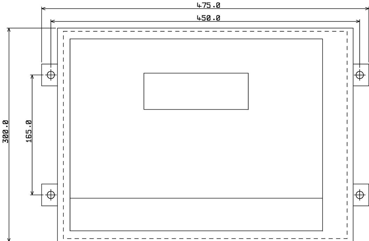
**Note:** The front panels of the MCU control units open to allow access to the screw terminals situated inside. Sufficient space should be allowed around the mounting position so that this action is not restricted.
