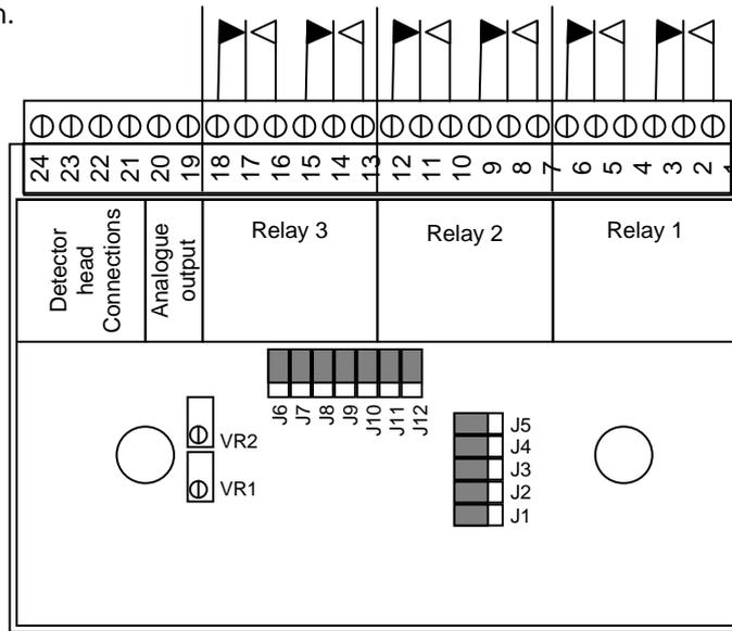
The relay connections shown are with the relay coil in its de-energised state.
