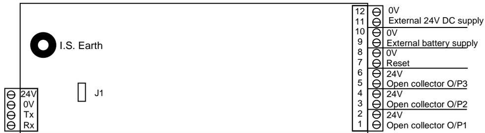
The lower 4-way connector provides a 24V and 0V connection. The voltages are always present at these terminals whilst FS2 is intact. The remaining two connections must not be used. The 24V supply is designed for use by Analox Ltd when powering external equipment. The amount of power available from this connector must be determined for each installation based upon the system configuration.
