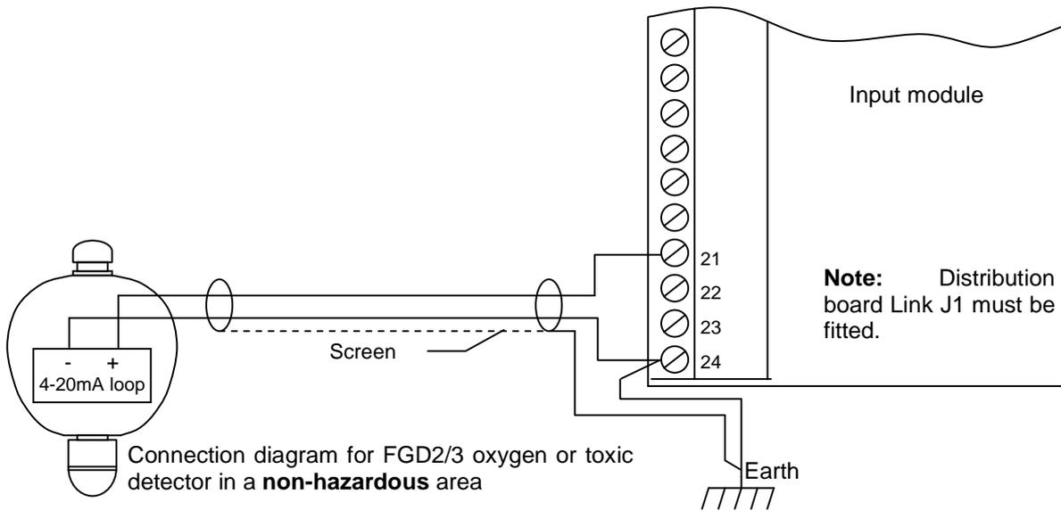
The correct wiring method for all Analox Ltd FGD2 / FGD3 detector heads (in a non-hazardous location) is shown above. It is important to note that this drawing shows the wiring connections but does not discuss the input module configuration. Prior to connecting the detector head ensure the input module is correctly configured (refer to section 4.1).
