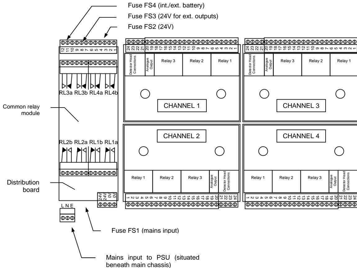
The diagram above shows a pictorial representation of the various module positions within the MCU3 and MCU4 Control Units.
